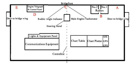
Figure 2: Crimson Mars's bridge layout with details relevant to the incident
