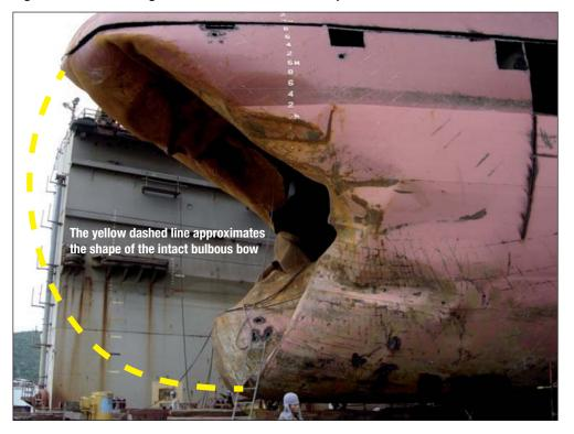
Figure 5: The damaged bulbous bow seen from the port side
