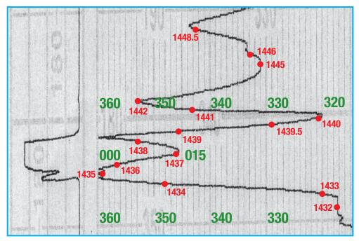
Figure 9: Section of course recorder chart enlarged and expanded
