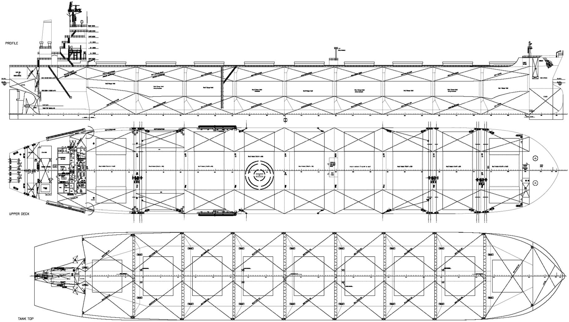
Figure 3: *Flash* General Arrangement Plan
