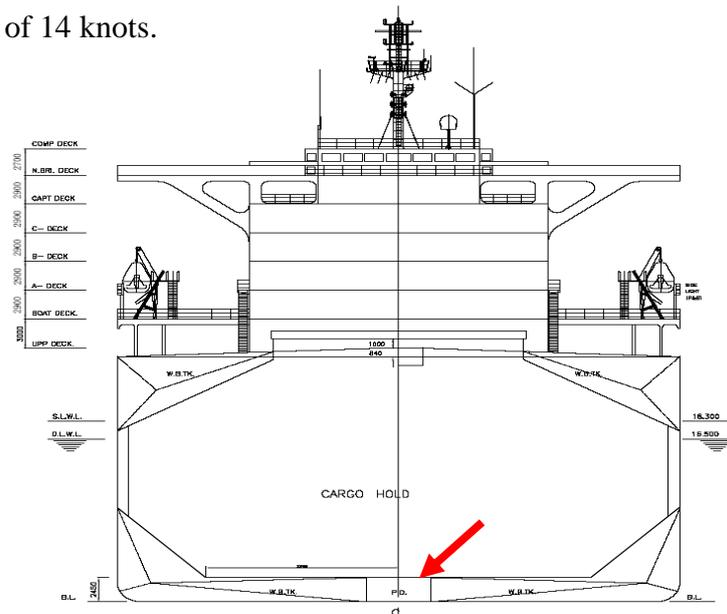
Figure 2: Duct keel running almost the entire length of the vessel, to the engine-room's forward bulkhead
