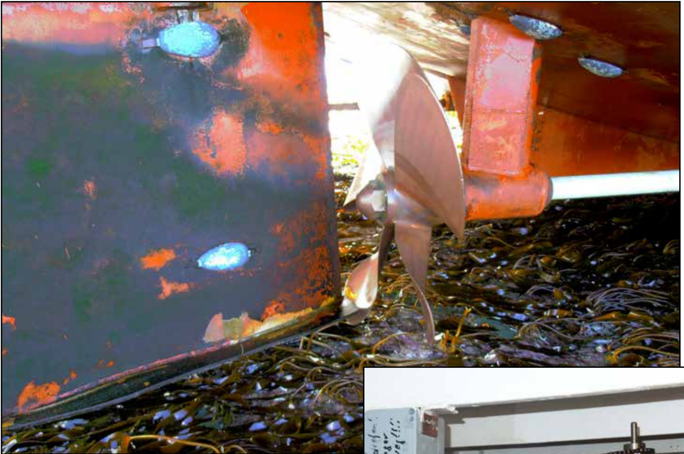
Figure 3: Damage to starboard propeller and rudder (inset: internal damage)
