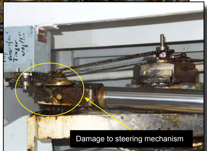
Figure 3: Damage to starboard propeller and rudder (inset: internal damage)
